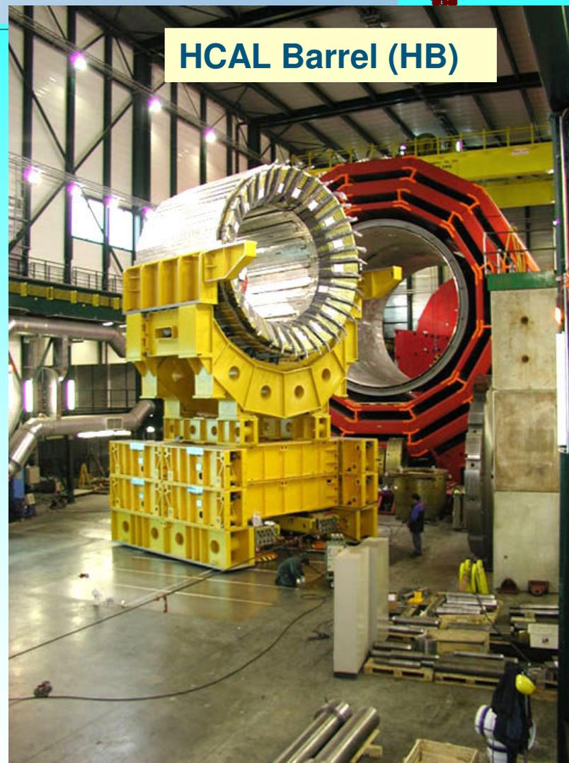
Assembly of 2 half barrels HB+ & HB- and two endcaps HE+ & HE- completed in 03 (brass+ scint)
