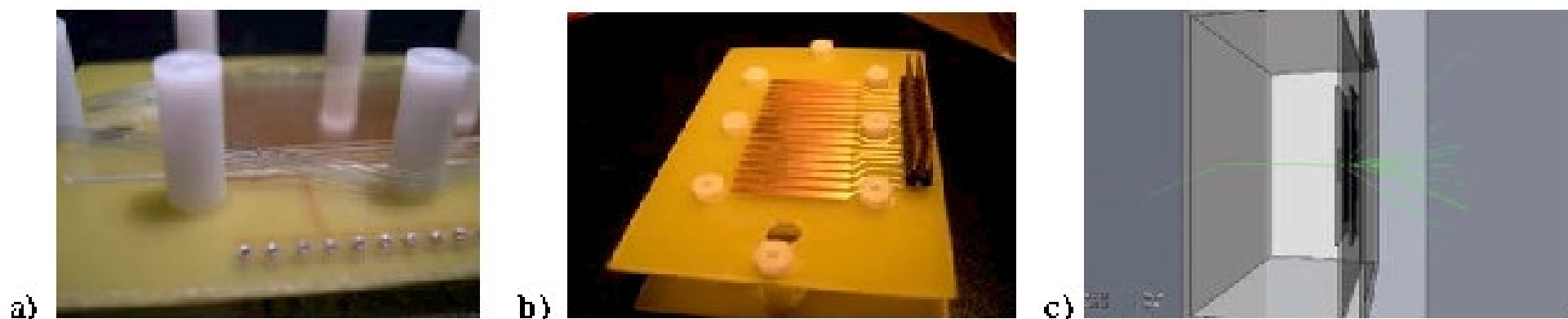
Fig. 5. a- glass MRPC prototype being assembled; b- 2 mm readout strips facing the detector; c- visualization of simulated tracks in aluminium case.
